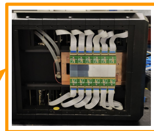
TimePix3 (Si-based detector for beam monitoring)
