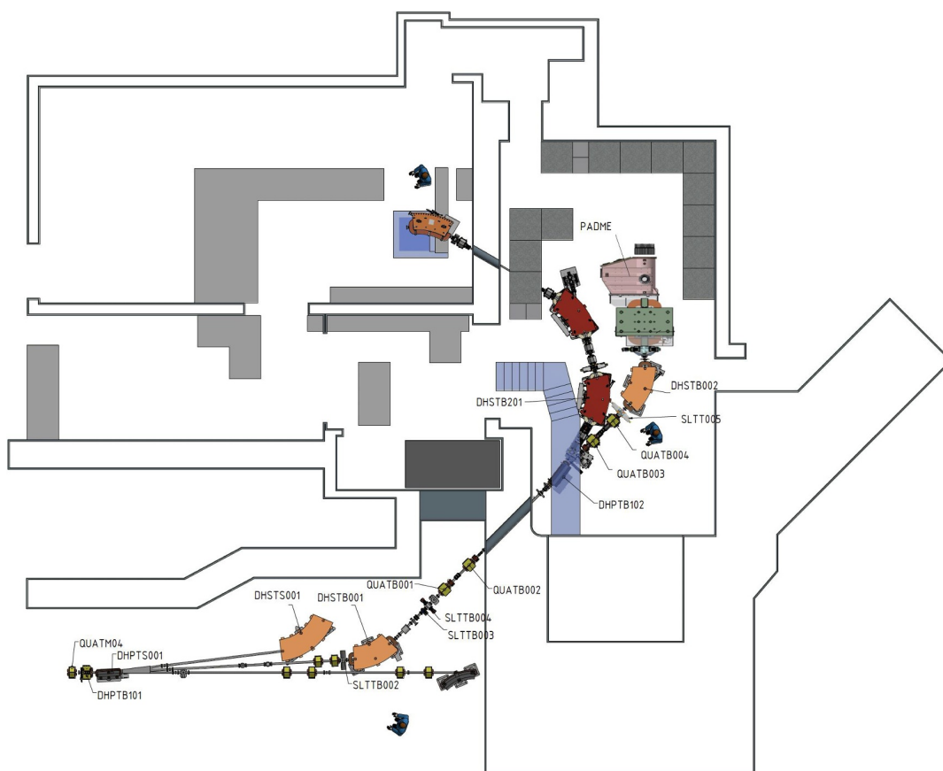
Figure 1. Sketch of the PADME beam line and the BTF-1 complex at LNF.
