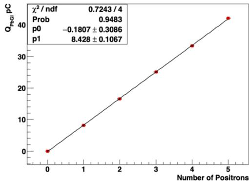
Figure 17. Fit to the single particle response.
