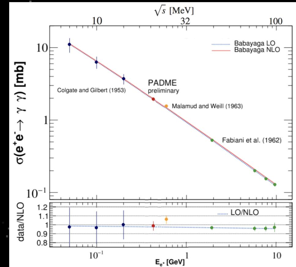
$$\sigma(e^+ e^- \rightarrow \gamma\gamma) = (1.977 \pm 0.018_{\text{stat}} \pm 0.118_{\text{syst}}) \text{ mb}$$
