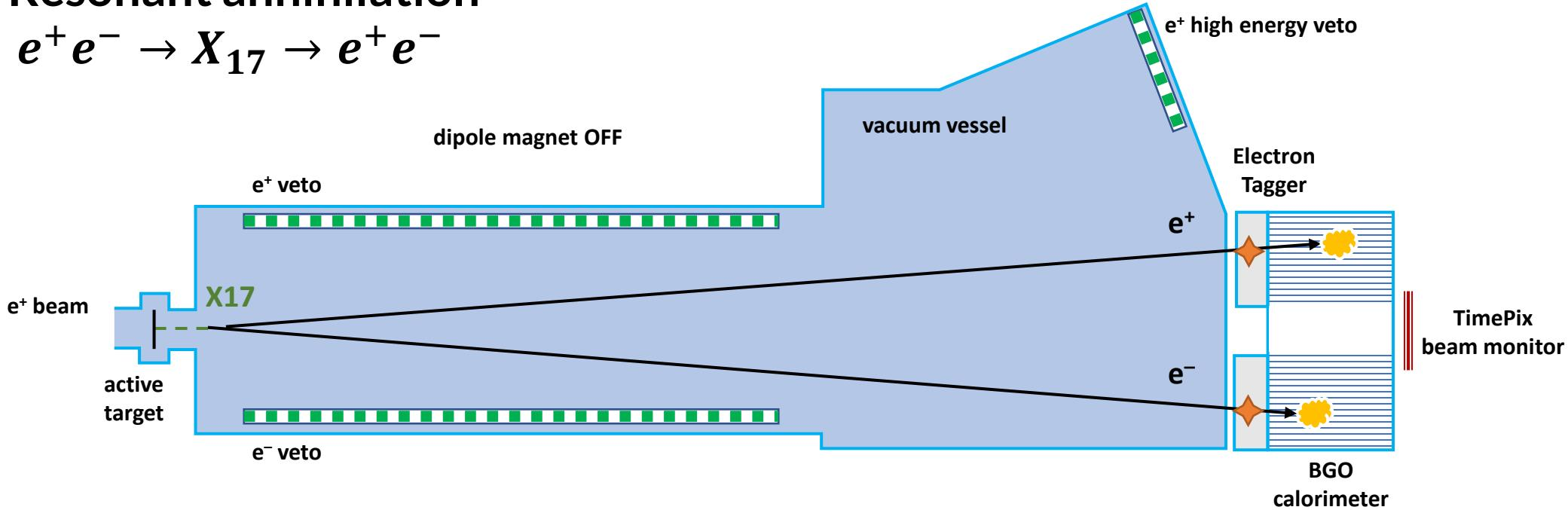
Different detector setup: magnet off, no SAC, TimePix on beamline, Electron Tagger in front of BGO
