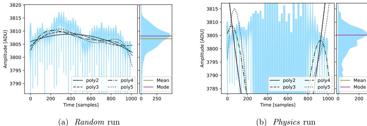
**Figure 2.** 5000 events ADC 27, channel 12, capacitor 16. The width of the violins represent the population at a given amplitude.
