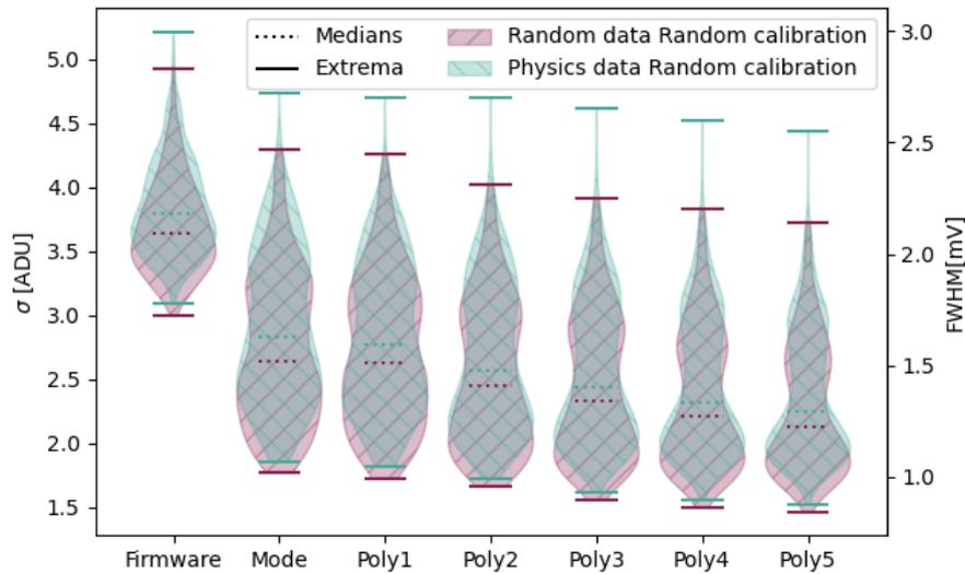
**Figure 3.** Comparison between different calibration methods. To obtain this plot 5000 events were used from both *Random* and *Physics* runs. Channels 16-24 of ADC27 are excluded from the statistics as they are known to be noisier.
