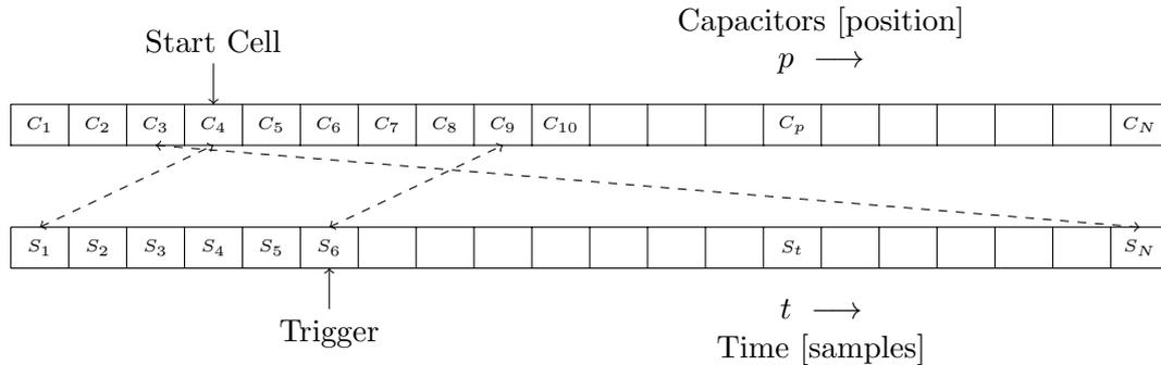
**Figure 1.** Illustration of the relationship between capacitors and time positions. The lower row represents samples  $S$  in time, while the upper one represents the capacitors in the circular buffer.
