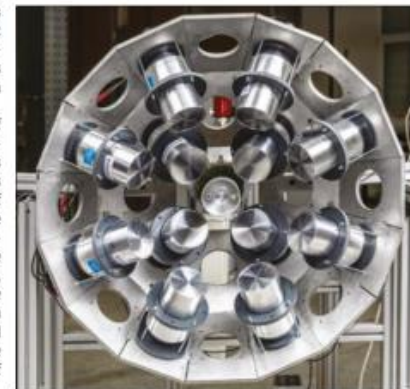
Future view Atomki's new high-resolution LaBr 3 spectrometer, which will record gamma-gamma pairs from excited nuclei.
