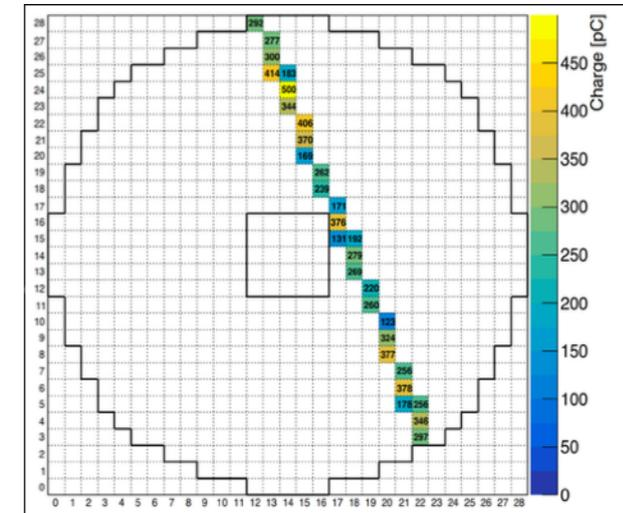
ECAL 1  $\mu\text{s}$  window, 1GHz sampling
