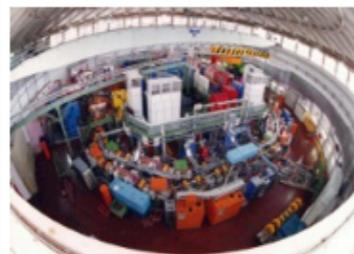
The LINAC of the DAΦNE complex provides a positron beam for a fixed target experiment: PADME
