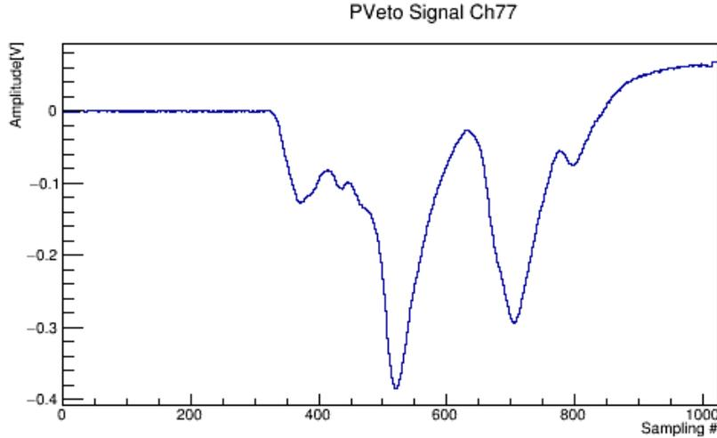
**Figure 3.** Example of a PVeto signal for a random channel after pedestal subtraction.
