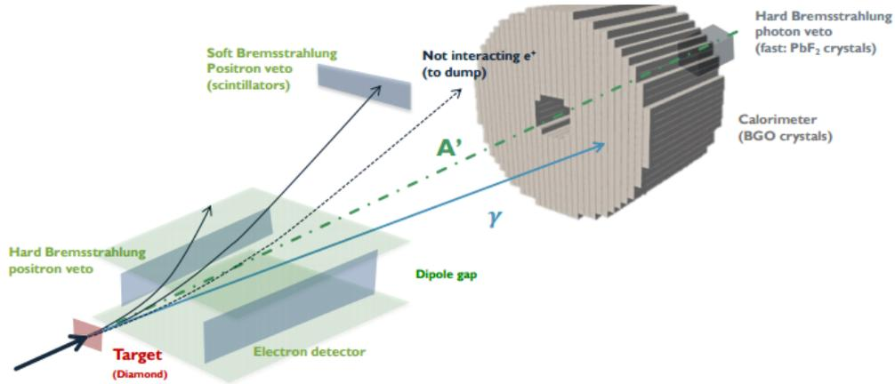
**Figure 1.** Layout of the PADME detector. The positron beam of energy up to 550 MeV hits the target. The signal is represented by a cluster in ECAL due to a single SM photon, emitted in coincidence with a dark photon. The non-interacting beam goes to the beam dump; SM physics processes like the annihilation in two (or three) photons and Bremsstrahlung are the main source of background.
