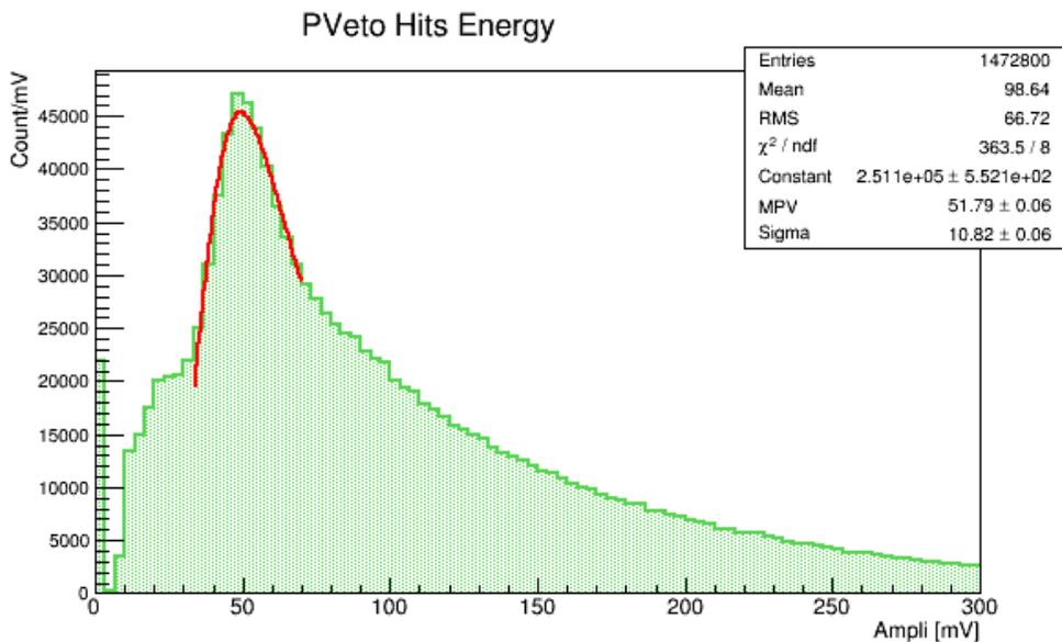
**Figure 4.** Positron Veto signal pulse height distribution for 10000 events. A Landau fit is superimposed, which gives a Most Probable Value of about 51.8 mV.
