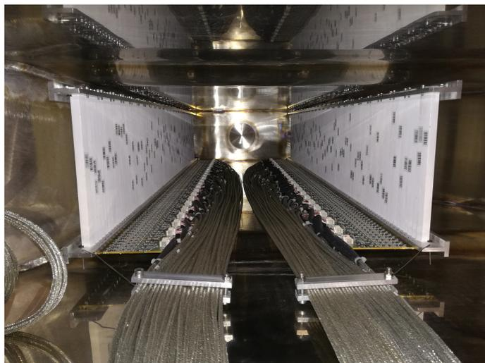
**Figure 2.** View of the internal vacuum chamber, just before the final assembly. The EVeto (on the left) and the PVeto (on the right) are shown. The beam comes from the front.
