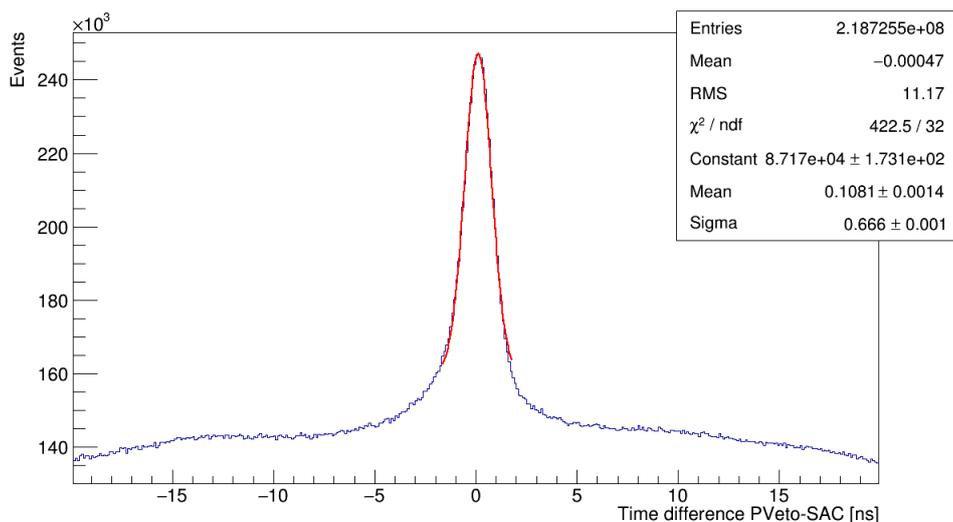
**Figure 5.** Time difference between the PVeto hits and the hits of a single SAC central crystal. The sigma value of the gaussian fit superimposed gives an estimate of the time resolution ( $\sigma_t \simeq 670$  ps).
