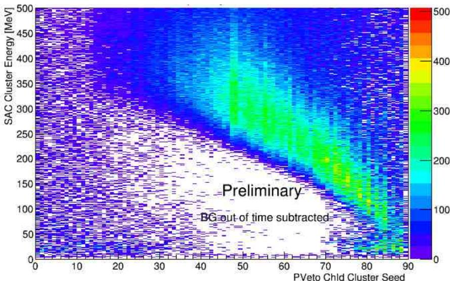
**Figure 6.** SAC cluster energy as a function of the PVeto cluster position for  $\Delta t < 1 \text{ ns}$ . A clear correlation between the SAC cluster energy and the Channel Id of the cluster seed, proportional to the Z position of the PVeto in the PADME frame, is shown. Beam energy 490 MeV, 11M POT.
