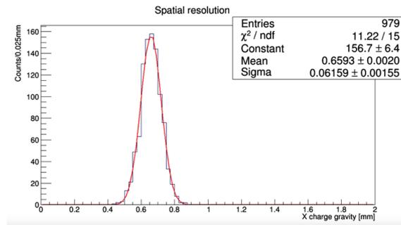
**Figure 3.** Spatial resolution of the target.
