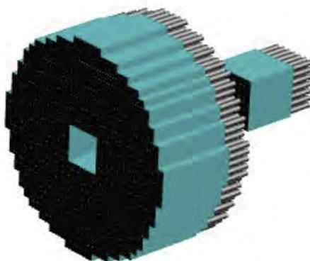
**Figure 4.** Outline of the calorimeters. The larger ECAL is upstream the beam, with a hole in the central part. The SAC is placed on the back, to detect the photons entering the hole.
