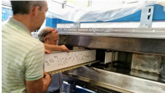
**Figure 3.17.** Picture during the installation of the PVeto and EVeto inside the vacuum chamber.
