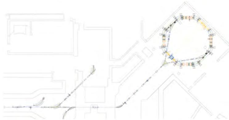
**Figure 3.2.** Layout of the transfer-lines from the end of the LINAC to the damping ring, with the original configuration of the line towards the Beam-Test Facility.
