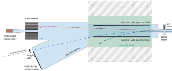
Fig. 1. – PADME detector layout. The distance between the target and the calorimeter (which has a radius of 29 cm) is 3 m, while the small angle calorimeter is a square of 14 cm side.
